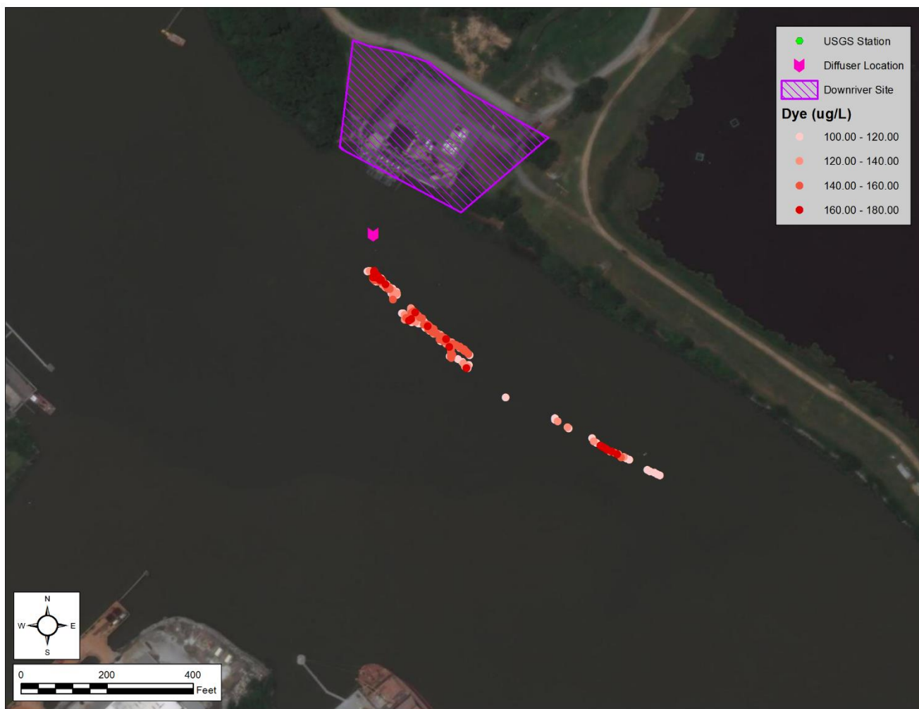
Figure 10-12 Front River Dye Sampling – August 25, 2020 (mid-depth) (100 to 180 µg/L)
