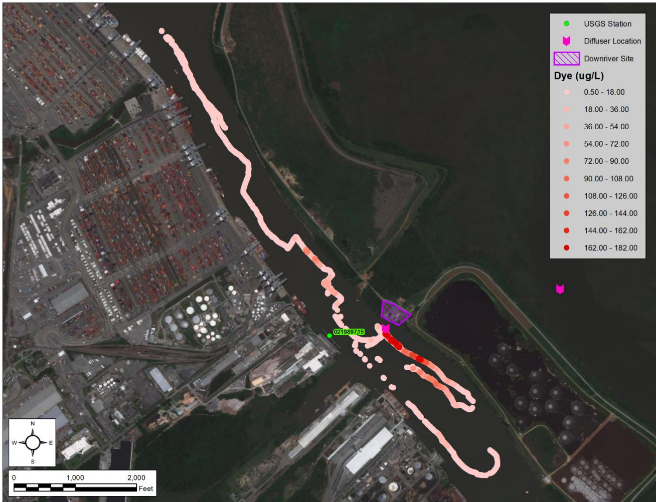
Figure 10-15 Front River Dye Sampling – August 25, 2020 (mid-depth) (100 to 180 µg/L)
